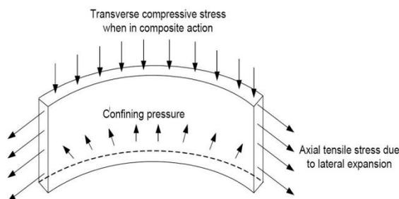
**Figure 1: Triaxial State of Stress in FRP**
