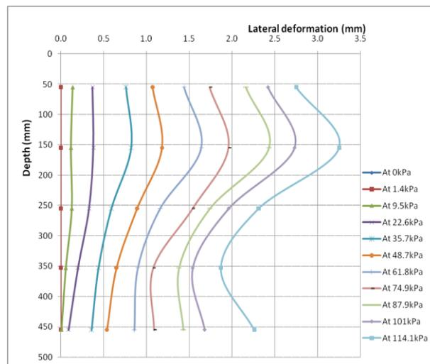
Figure 8. Vertical profile of geotextile reinforced wall loaded up to half the design surcharge at natural moisture content
