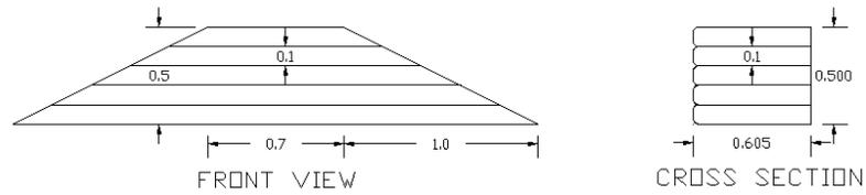
Figure1. Front and end view of the model vertical wall
