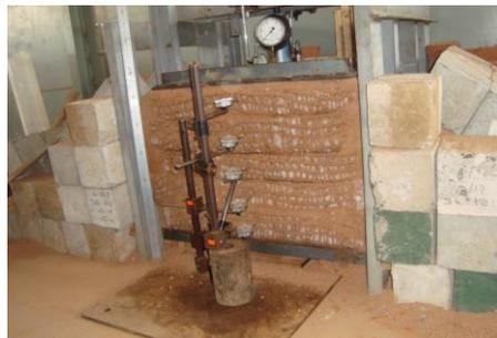
Figure 2. Arrangement of test set up for geo-mat reinforced wall
