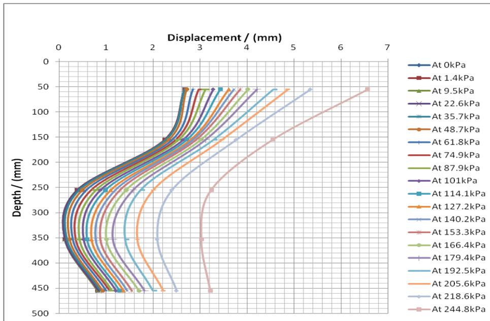
Figure 6. Vertical profile of coir geomat reinforced wall during the reloading stage at natural moisture content
