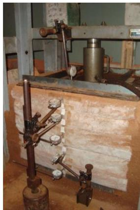
Figure 3. Arrangement of test set up for geotextile reinforced wall
