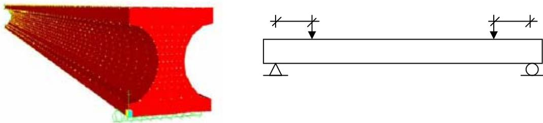
**Figure 3. 3D view of a model with circular voids and the loading arrangement**
