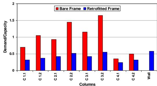
**Figure 15.** Demand-to-Capacity Ratio for the bare and wall-retrofitted frames
