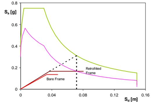
**Figure 5. Demand spectra and capacity curve in AD format at the LSSD for the frame retrofitted with FRP wrapping and R/C jacketing**
