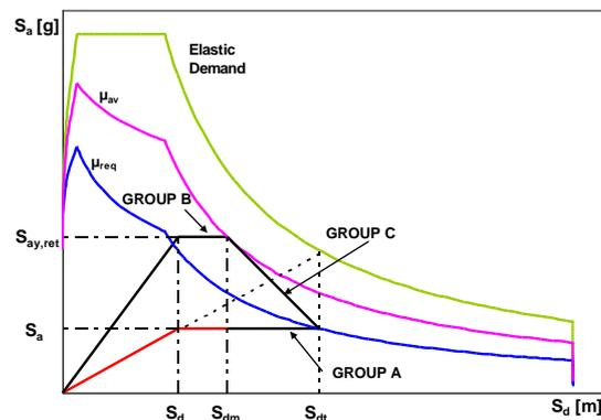
*Figure 1. Capacity curves for different retrofitting strategies*
