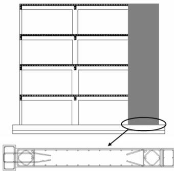
**Figure 12.** Elevation view of the retrofitted R/C frame and cross-section detailing of the infill wall
