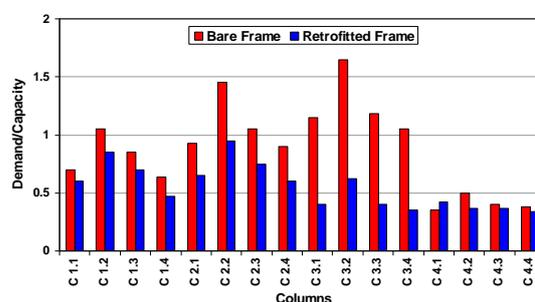
*Figure 7. Demand-to-Capacity Ratio for the bare and retrofitted frames*
