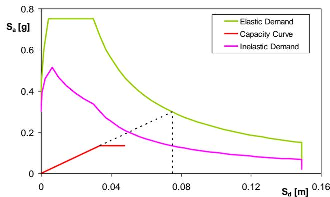
**Figure 3. Demand spectra and capacity curve in AD format at the LSSD for the bare frame**
