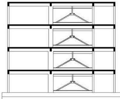
**Figure 8. Elevation view of the R/C frame retrofitted with eccentric steel bracing**
