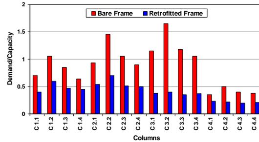
*Figure 11. Demand-to-Capacity Ratio for the bare and retrofitted frames*
