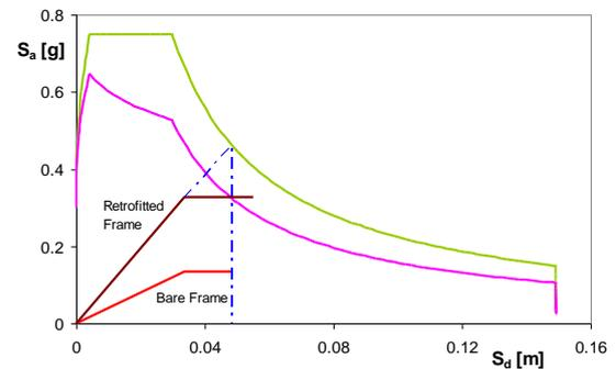
**Figure 9. Demand spectra and capacity curve in AD format at the LSSD for the frame retrofitted with eccentric steel bracing**
