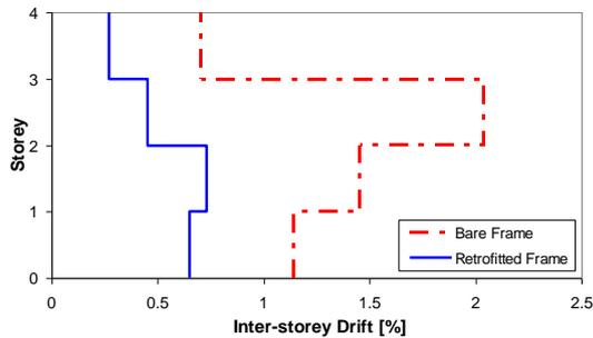
*Figure 10. Inter-storey drift profiles for the bare and retrofitted frames*
