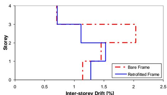
*Figure 6. Inter-storey drift profiles for the bare and retrofitted frames*
