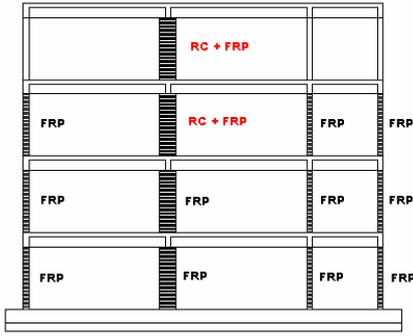
**Figure 4. Selective retrofitting intervention with FRP wrapping and R/C jacketing**
