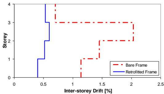
**Figure 14.** Inter-storey drift profiles for the bare and wall-retrofitted frames
