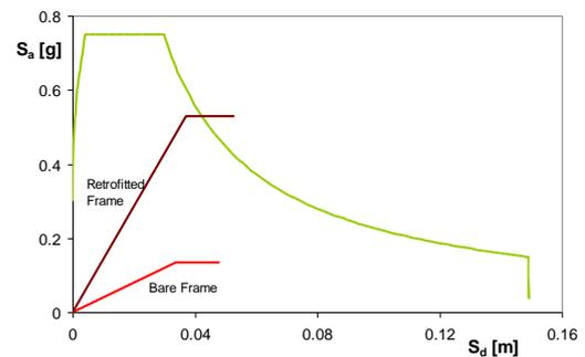
**Figure 13.** Demand spectra and capacity curve in AD format at the LSSD for the frame retrofitted with infill wall
