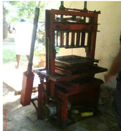
*Figure 4-Local block manufacturing machine*
