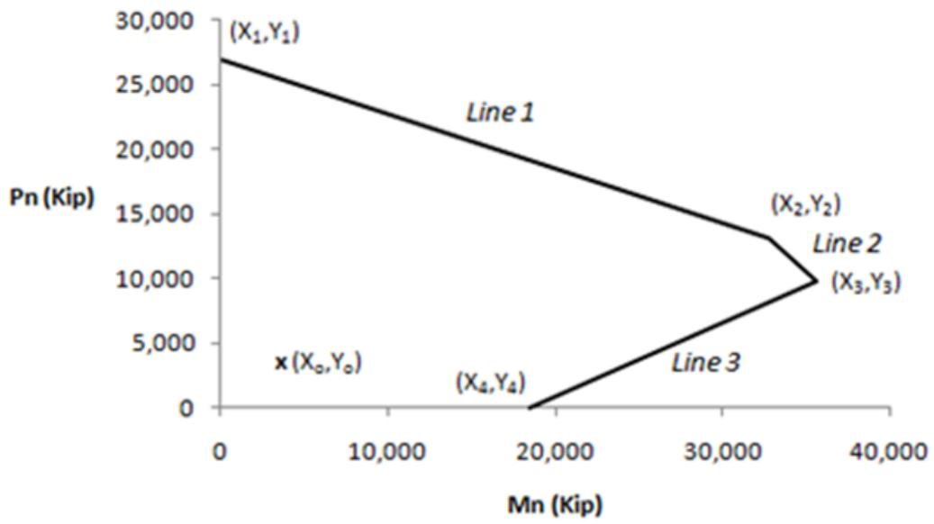
Figure 4: Interaction Diagram about X-X Axis
