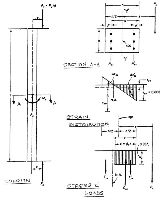
Figure 5: Cross Section, Strain Distribution, Stresses and Loads (Nawy, 2003)
