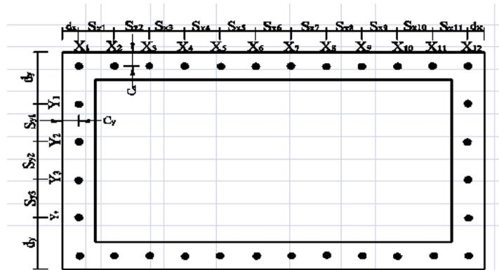
**Figure 3: Pre-stressing Strands and Rods in the Hollow segment**
