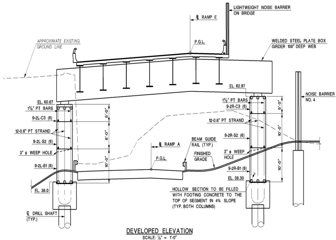
**Figure 1: General View of a Typical Pier**
