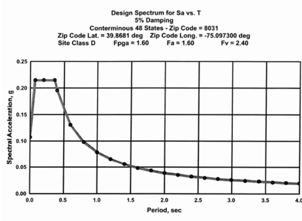
*Figure 2: Seismic Design Spectrum*
