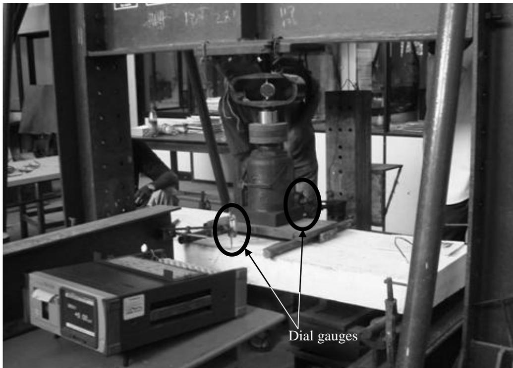
Figure 5: Test arrangement
