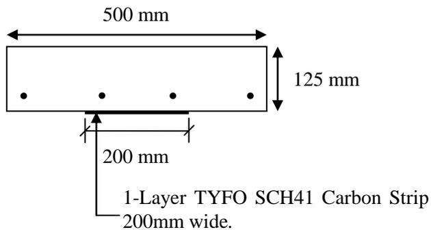
Figure 3: R6 – TS1 Cross section
