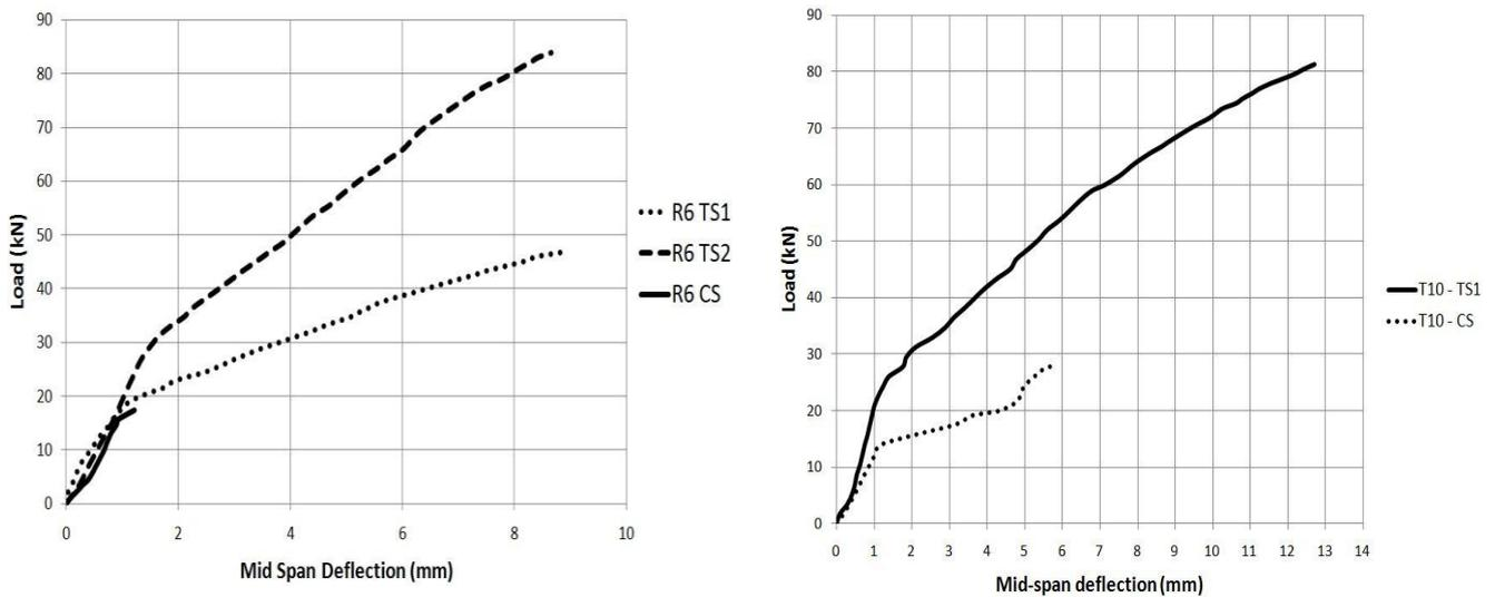
Figure 7: Load versus mid-span deflection relationship.
