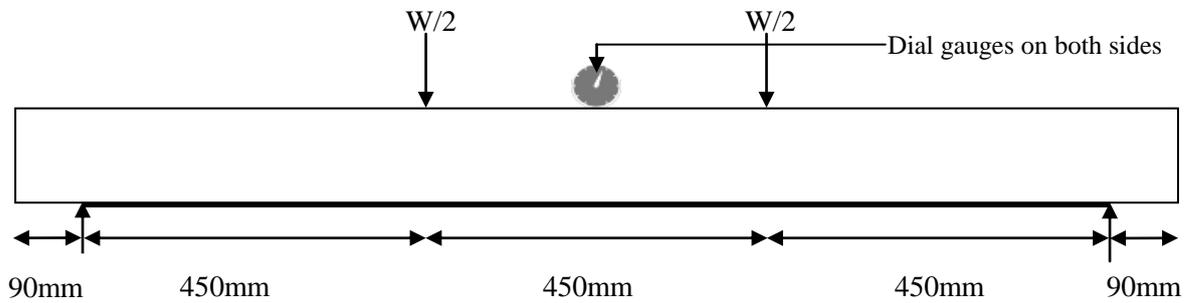
Figure 1: Slab loading pattern
