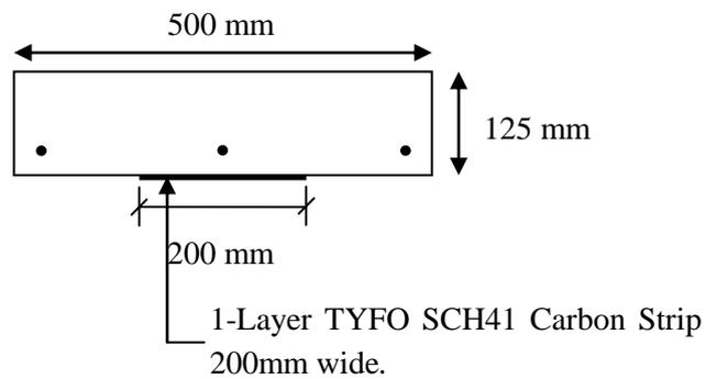
Figure 2: T10 – TS1 Cross section
