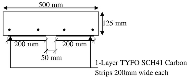
Figure 4: R6 – TS2 – Cross section
