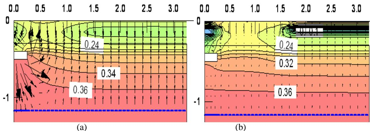
Figure 4. Predicted soil moisture content distributions around an absorption trench for a groundwater table depth of 1.2 m and wastewater loading rates of: (a) 5mm/day; (b) 0 mm/day
