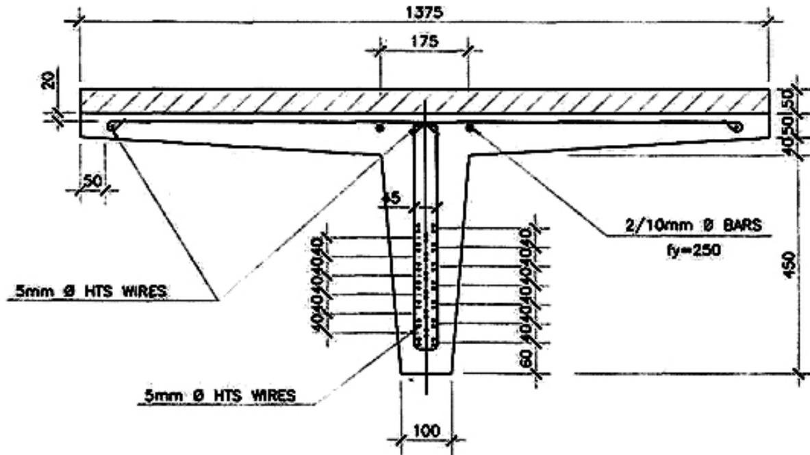
Figure 8: A section of the typical T-beam
