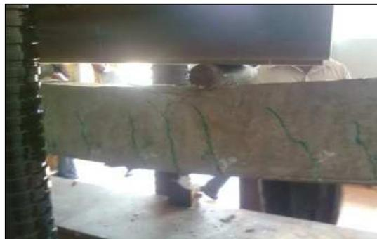
Figure 5: Flexural cracks of the control specimen
