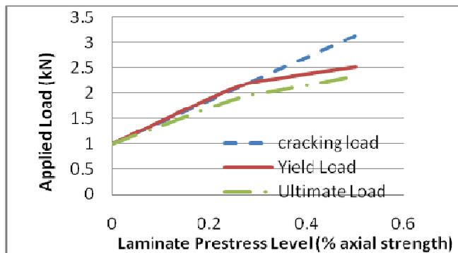
Fig.5 Normalized-Load Milestones Vs. Laminate prestress levels
