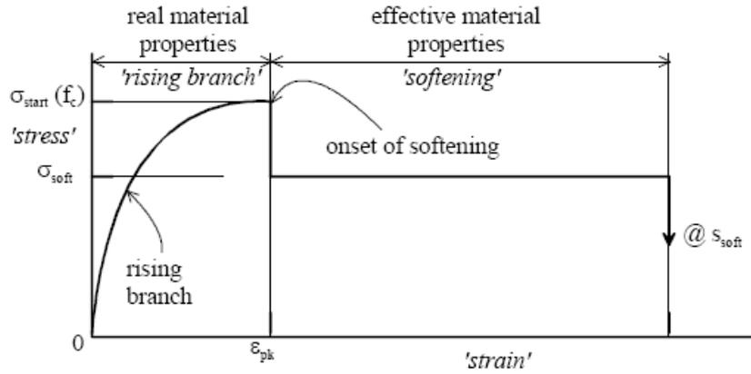
Fig.2 Stress strain relationship of concrete under compression
