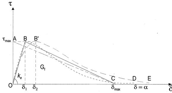
Fig.4 various interface bond characteristics
