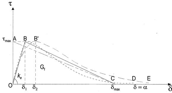
Fig.4 various interface bond characteristics
