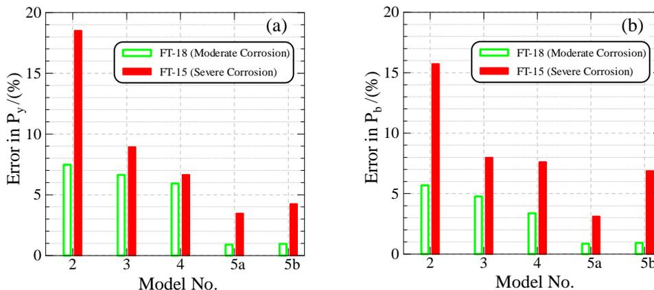
Figure 7: Comparison of %errors in (a) yield and (b) tensile strength estimation of different special analytical models
