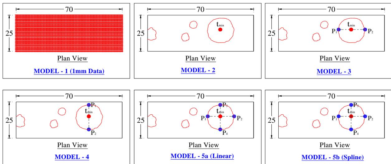
Figure 5: Analytical models with special corroded surface measurement points
