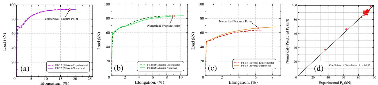
Figure 3: Comparison of experimental and analytical load-elongation curves of specimens with; (a) minor corrosion [FT-22], (b) moderate corrosion [FT-18], (c) severe corrosion [FT-15] and (d) comparison of experimental and analytical ultimate load capacities
