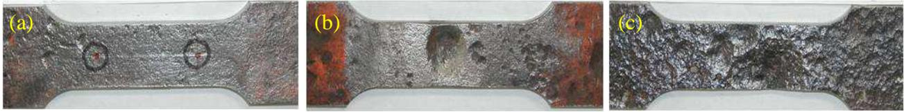
Figure 2: Plates with (a) minor corrosion [FT-22], (b) moderate corrosion [FT-18] and (c) severe corrosion [FT-15]
