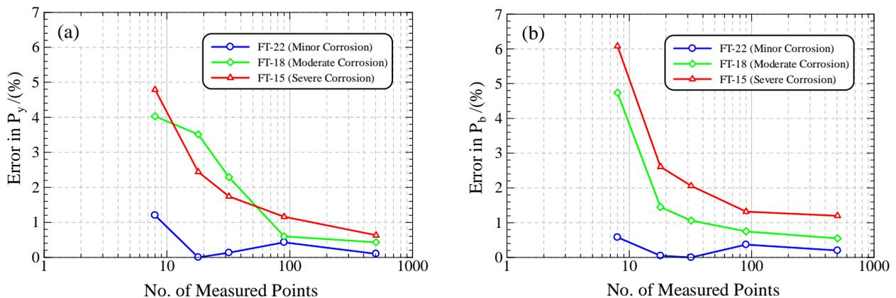
Figure 4: Comparison of %errors in (a) yield and (b) tensile strength estimation
