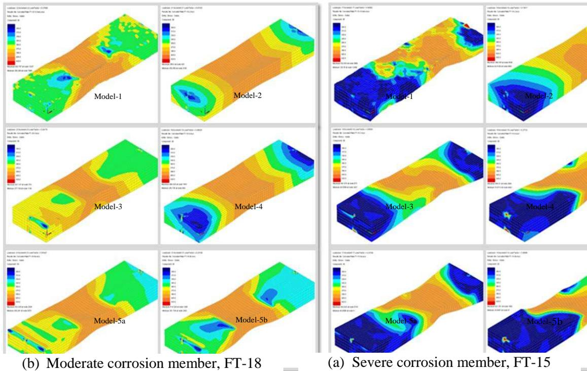
Figure 6: Stress distributions of different special analytical models at ultimate load
