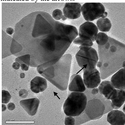
**Fig. 2** HRTEM image of gold nanoparticles obtained from the extract of resting cells exposed to 1 mM  $\text{HAuCl}_4$
