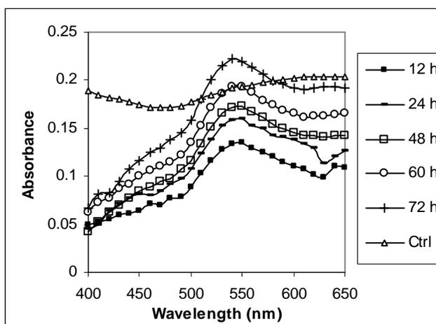
**Fig. 1** UV-visible spectrum of the extract obtained from resting cells of *Fusarium oxysporum*, exposed to 1 mM  $\text{HAuCl}_4$
