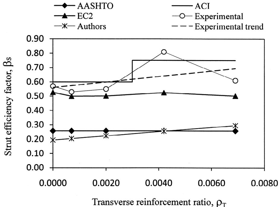
**Fig. 4** Trend in experimental and predicted strut efficiency factors with varying transverse reinforcement ratio (washed recycled aggregate concrete)
