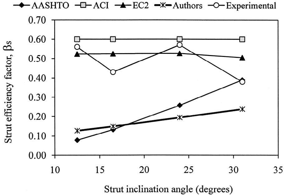
**Fig. 5** Trends in experimental and predicted strut efficiency factors with varying strut inclination (washed recycled aggregate concrete)
