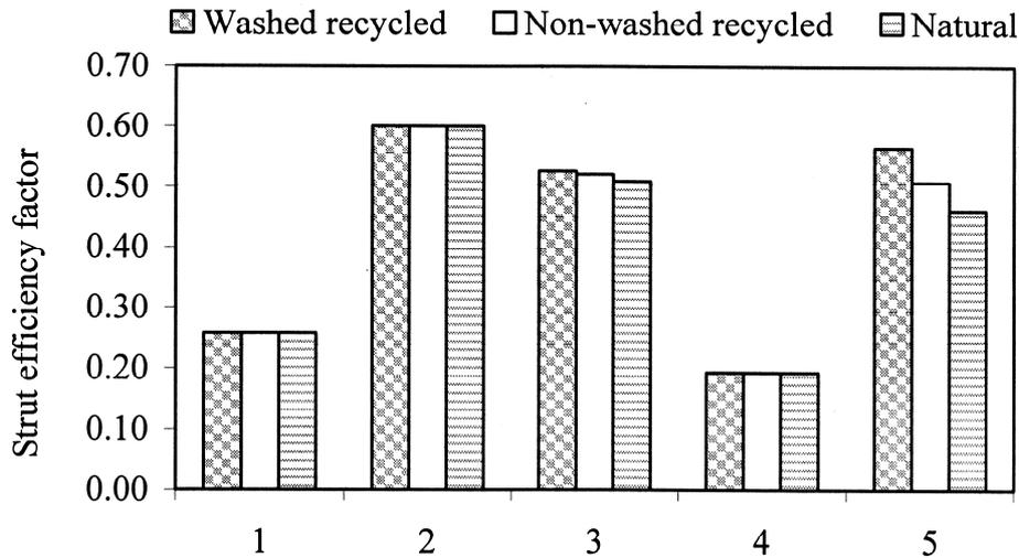
**Fig. 2** Influence of type of aggregates on the efficiency factor of bottle-shaped struts without transverse reinforcement [1. AASHTO, 2. ACI, 3. EC2, 4. Authors, 5. Experimental]
