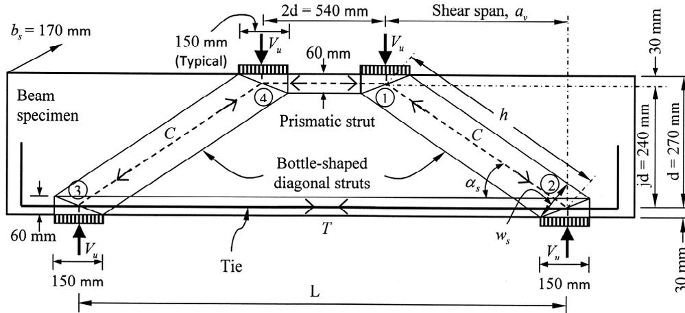
**Fig. 1:** Dimensions of a typical beam specimen with strut-and-tie model
