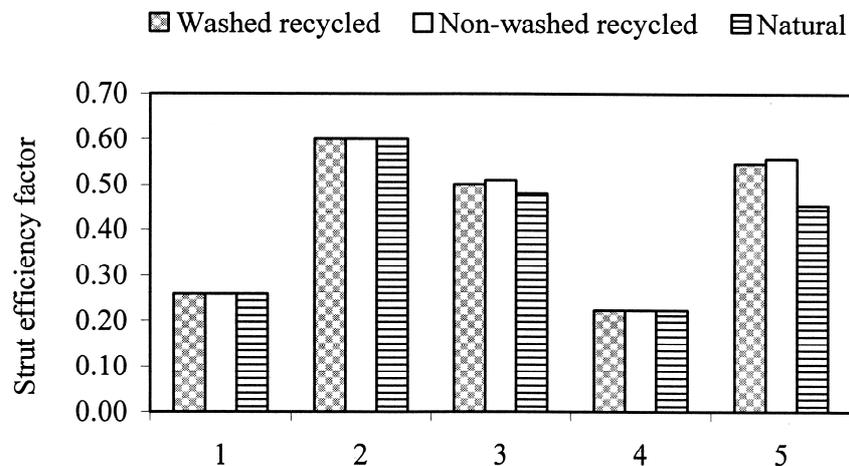
**Fig. 3** Influence of type of aggregates on the efficiency factor of bottle-shaped struts with 0.2% transverse reinforcement [1. AASHTO, 2. ACI, 3. EC2, 4. Authors, 5. Experimental]
