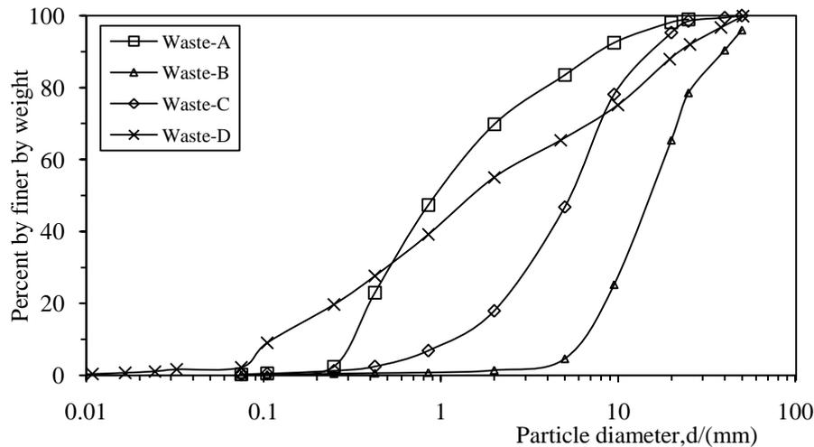
Fig. 1: Particle size distribution of different waste samples.
