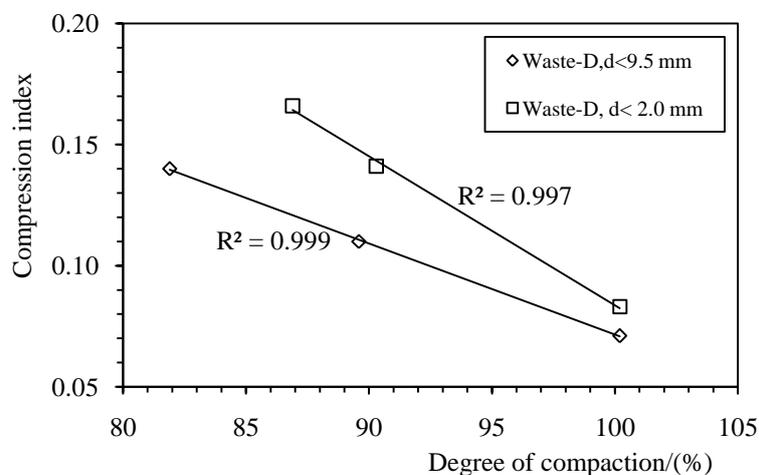
**Fig. 4: Change of compression index with the degree of compaction for Waste-D.**
