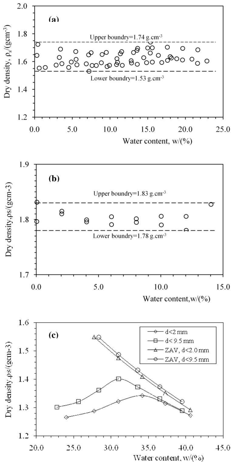
**Fig. 3: Moisture-dry density relationships: (a) Waste-A, (b) Waste-C, and (c) Waste-D. Zero air void lines are also shown**
