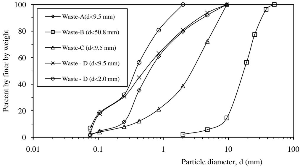
**Fig. 2: Particle size distribution of test samples.**
