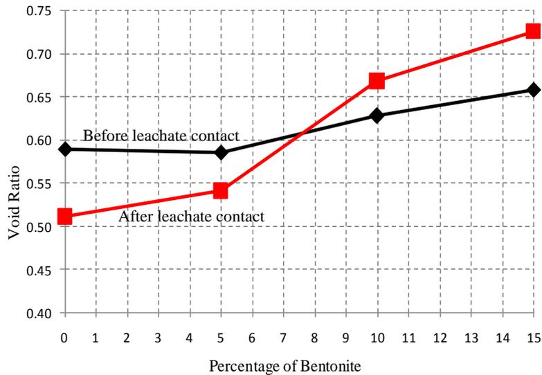
**Figure 6 – Variation of void ratio with the addition of bentonite**
