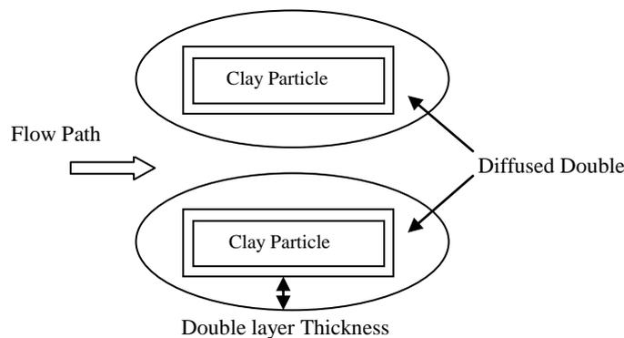
**Figure 5 – Reduction of hydraulic conductivity due to increase of double layer**
