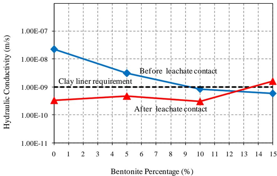
**Figure 4 – Variation of hydraulic conductivity with bentonite percentage**
