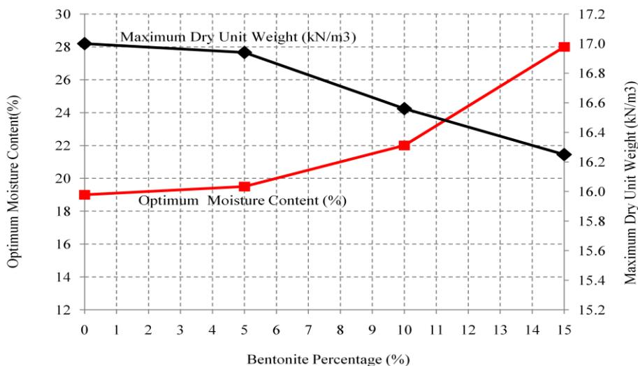
Figure 3 – Variation of compaction characteristics over bentonite content
