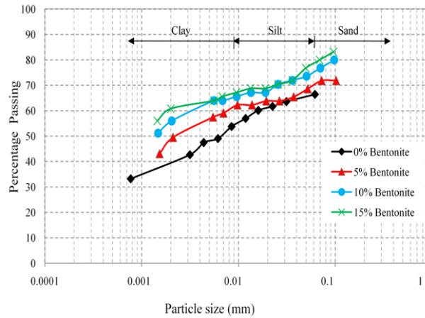
**Figure 1 – Particle size distribution of soil-bentonite mixtures**
