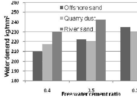
Figure 8 The increasing water demand with the increasing w/c ratio for 80% fine aggregate proportion.
