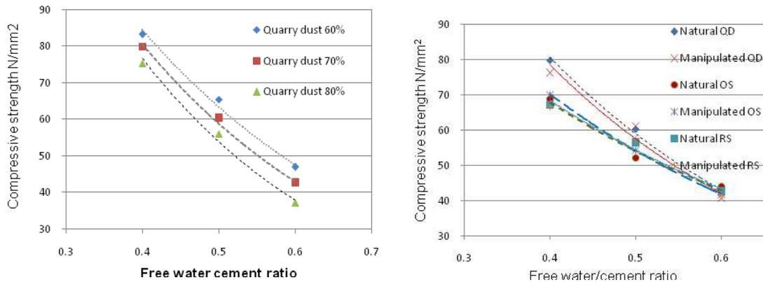
**Figure 9 Strength vs. water cement ratio for different proportions of quarry dust**      **Figure 10 Strength vs. water cement ratio for different particle size distributions**
