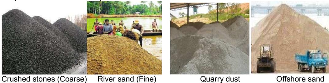
**Figure 4 Aggregate for concrete**
