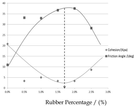
Figure 1: Variation of Cohesion and Friction angle with rubber content
