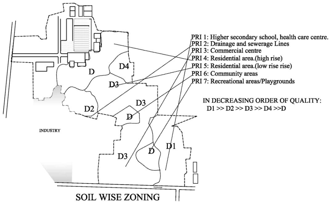
Figure 5: Soil specific Site Plan zoning
