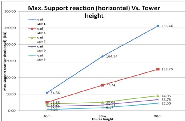
**Figure 4 – Variation of Support reactions (Horizontal)**
