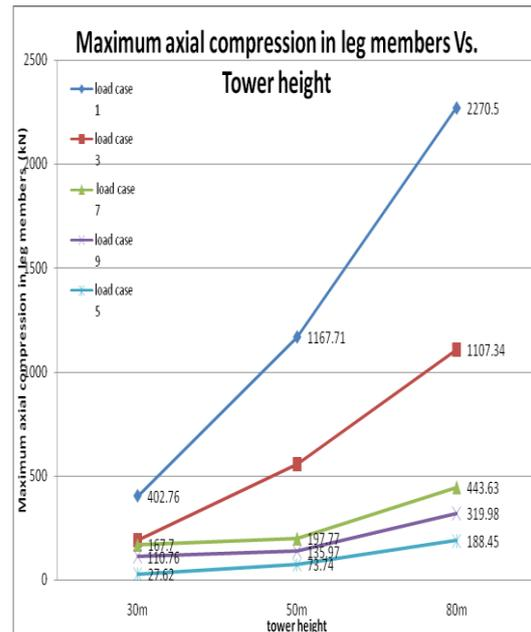
**Figure 7- variation of max. Axial compression in leg members**
