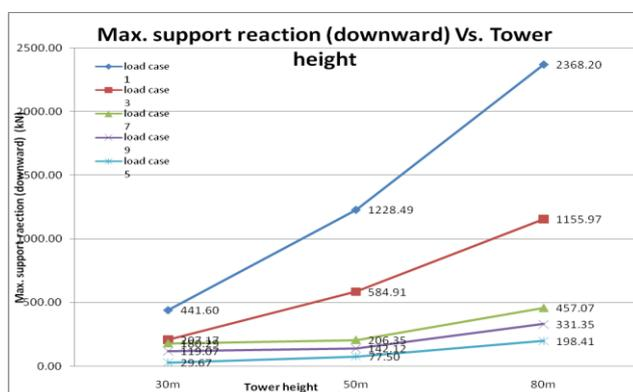
Figure 3 – Variation of Support reactions (Downward)
