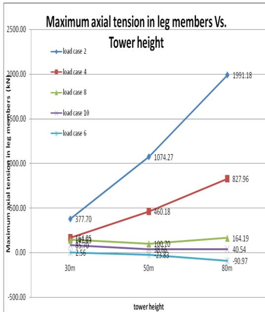
**Figure 6- variation of max. Axial tension in leg members**
