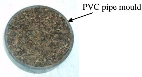
*Figure 2- Specimen used for noise testing*
