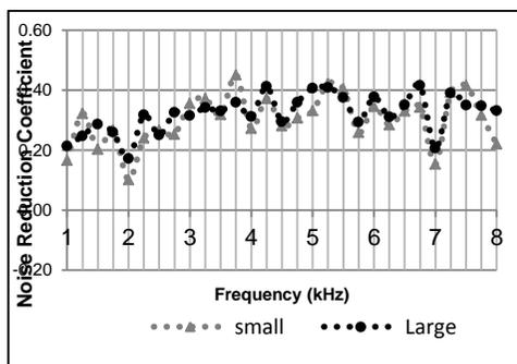
**Figure 6: Variation of NRC with particle size**
