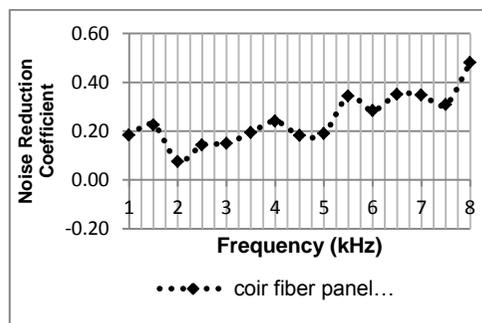
**Figure 7: NRC of Coconut coir fiber panel**
