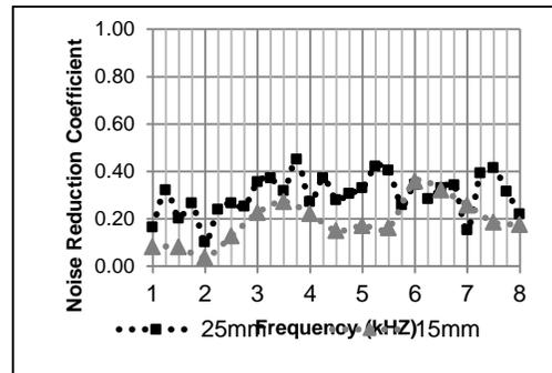
**Figure 5: Variation of NRC with tile thickness**
