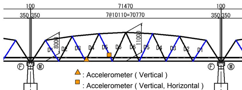
Figure 2 Positions of accelerometers in Measurement 2
