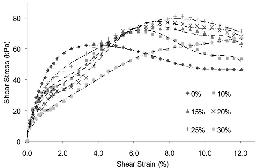
**Figure 2: Typical plot of variation of shear stress with shear strain for 5.6 mm crumb size with different percentage of rubber mix at normal stress of 100 kN/m<sup>2</sup>**
