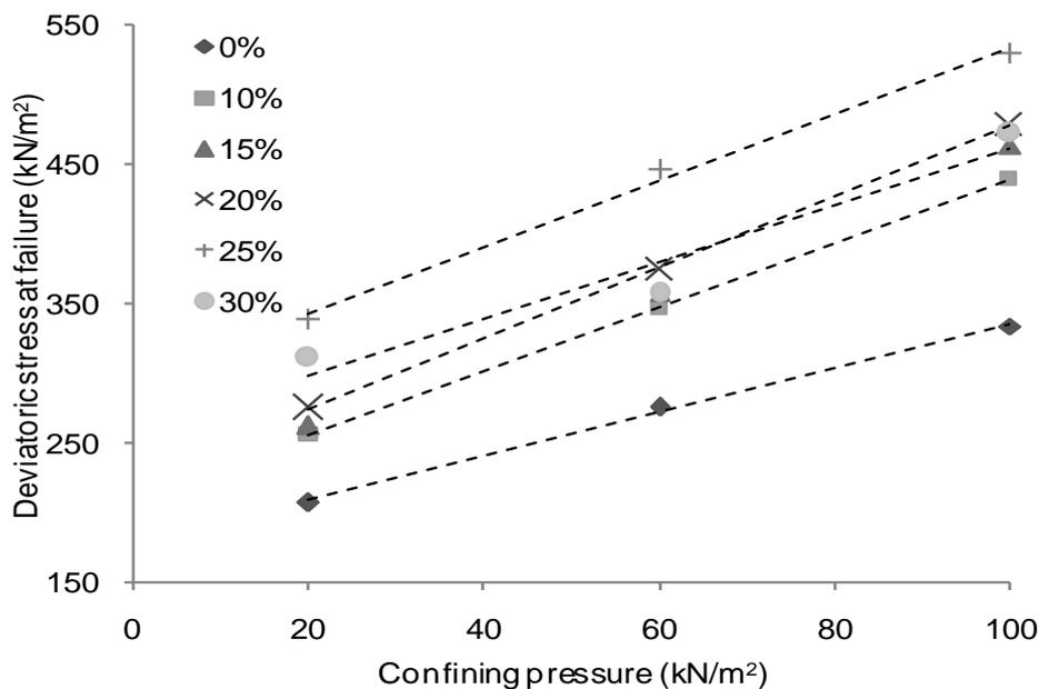
Figure 7: Effect of 5.60 mm rubber on deviatoric stress at failure for different composition
