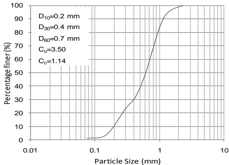
*Figure 1: Particle size distribution curve*
