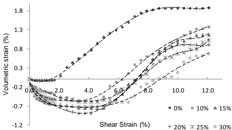
**Figure 3: Typical plot of variation of volumetric strain with shear strain for 5.6 mm crumb size with different percentage of rubber mix at normal stress of 100 kN/m<sup>2</sup>**
