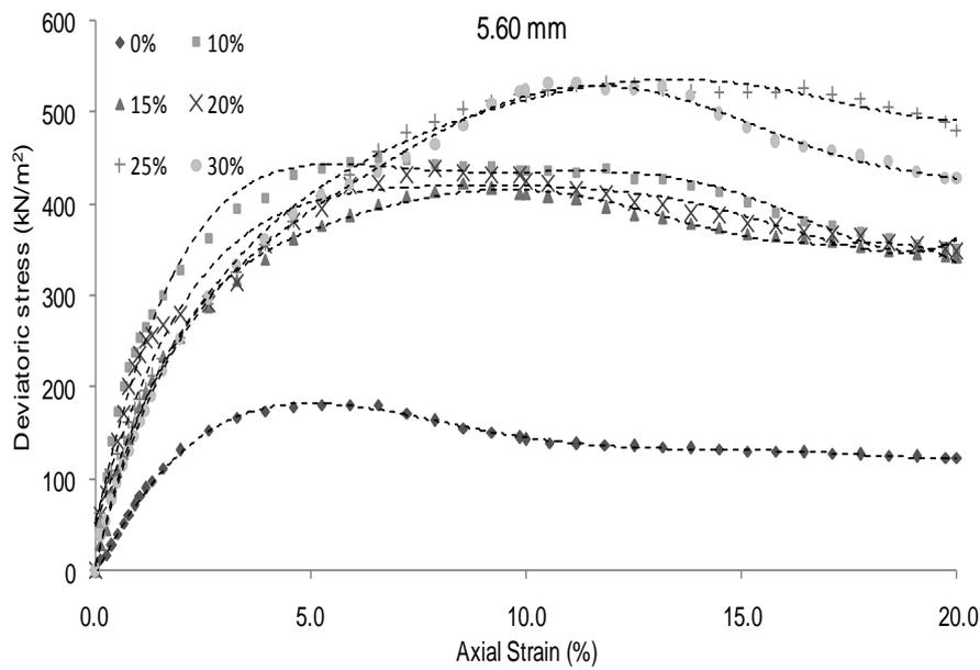
Figure 6: Stress-strain curves for confining pressure of 100kN/m<sup>2</sup> for different rubber size: (a) 1.00 mm, (b) 5.60 mm
