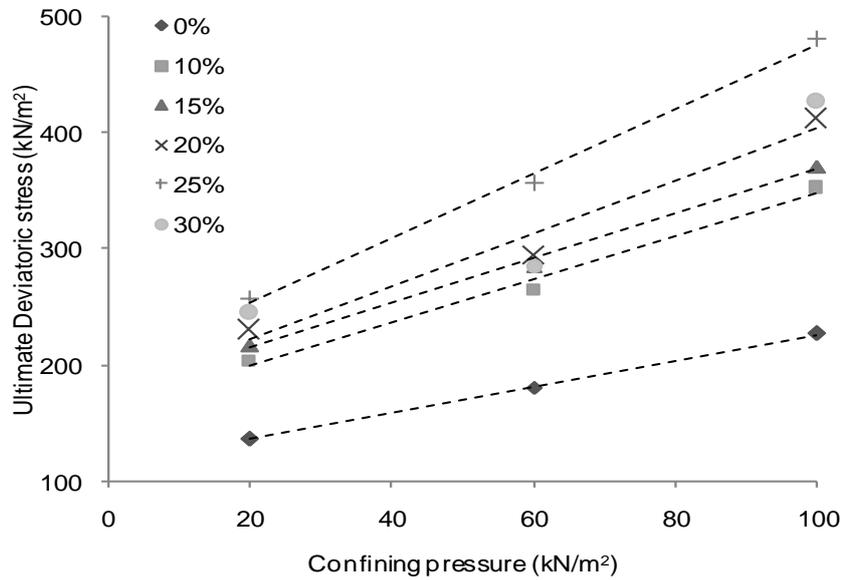
**Figure 8: Effect of 5.60 mm rubber on ultimate deviatoric stress for different composition**
