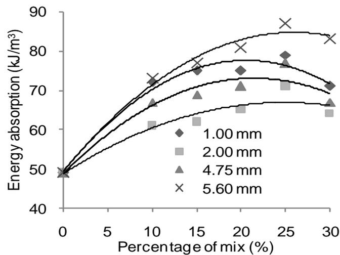
*Figure 10: Typical plot of variation of energy absorption capacity of sand with inclusion of rubber for confining pressure of 100 kN/m<sup>2</sup>*
