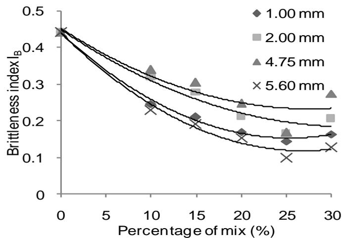
**Figure 9: Typical plot of variation of brittleness index of sand with inclusion of rubber for confining pressure of  $100 \text{ kN/m}^2$**
