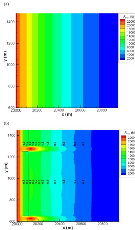
**Figure 5.  $x$ - $y$  distribution of the maximum tsunami force for (a) no-vegetation condition, (a) behind the forest for with-vegetation condition**
