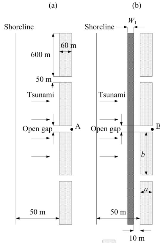
Figure 3. Schematic views of (a) exiting condition, (b) modified system
