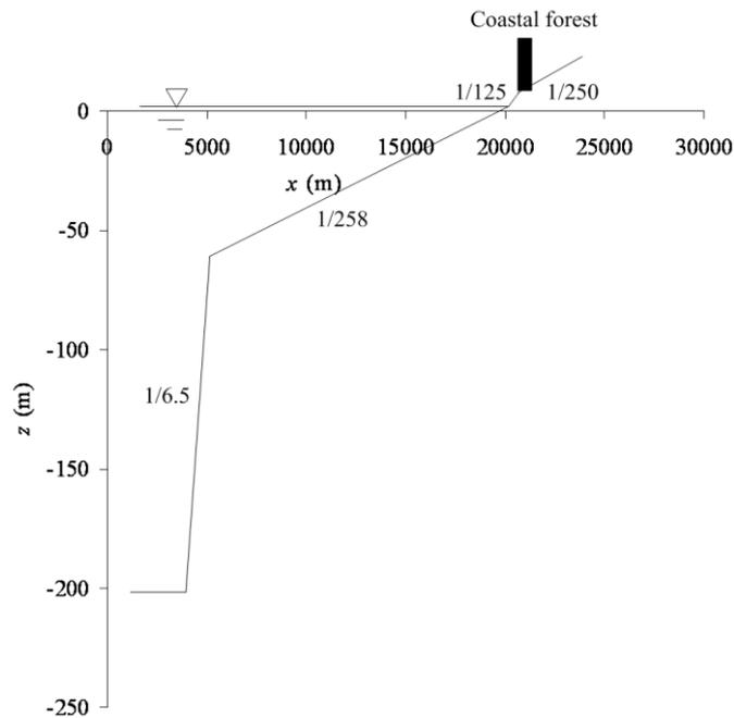
*Figure 2. The topographical conditions used for the numerical simulation*
