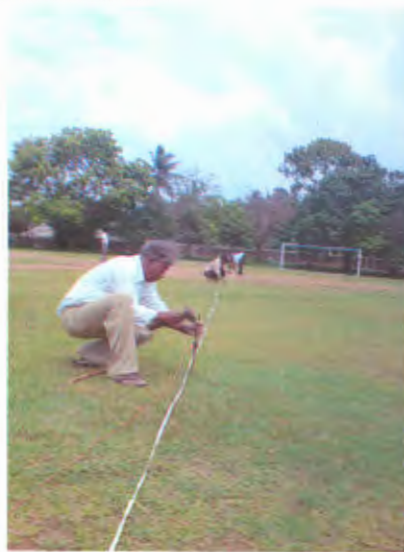
Figure 8.30 - (a) Spike connection to earth (b) changing array spacing along the field line (Original is in Color)
