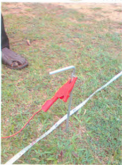
Figure 8.30 - (a) Spike connection to earth (b) changing array spacing along the field line (Original is in Color)
