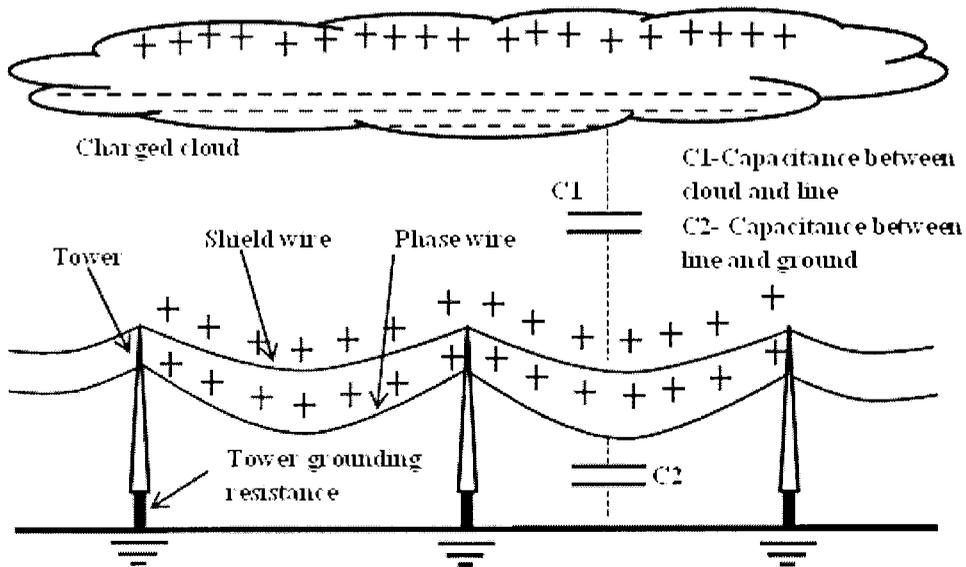
Figure 1.5 – Induced charges on a power transmission line
