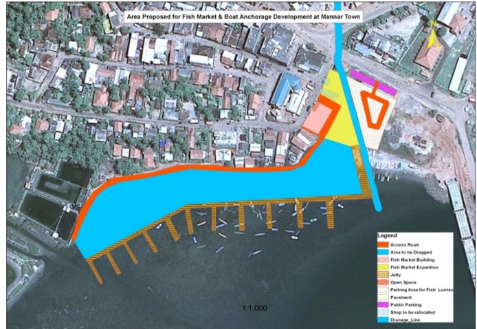
Fig 7: Redevelopment of foreshore area as a commercial and leisure precinct to include the redevelopment of the fisheries harbour, jetty with anchorage for 300 boats, modern fish market, restaurants and cafes and walkways
