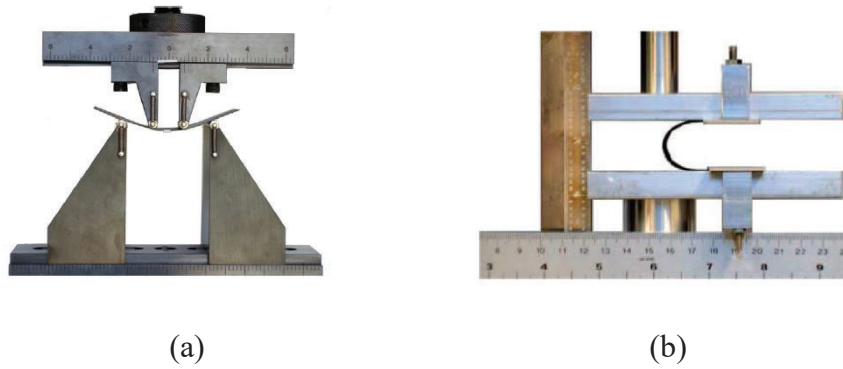
Figure 2.6 (a) Four-point bending test (b) Platen folding test (Mallikarachchi, 2019)
