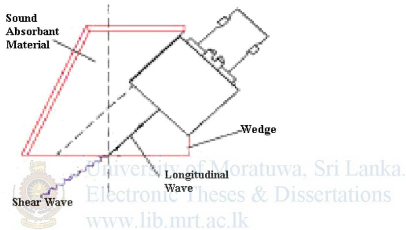
Figure 33: Cross section an angle beam probe<sup>45</sup>
