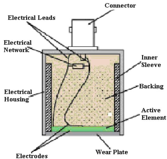
Figure 32: Cross section of typical contact transducer
