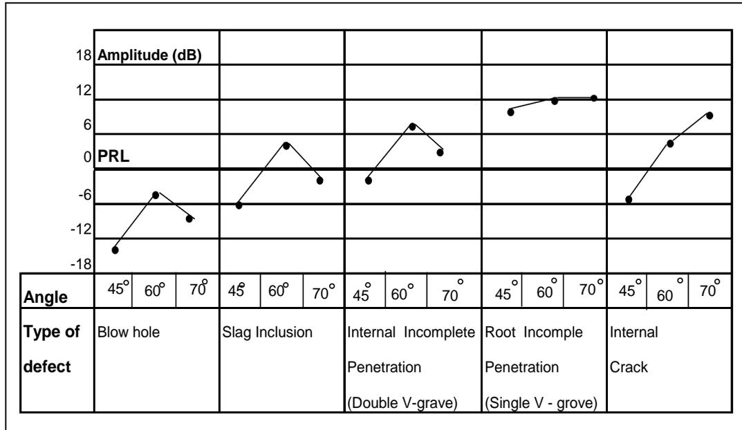
Figure 5: Graphical correlation between defect type,echo amplitude and angle of probe<sup>6</sup> (Thickness: 25 - 28 mm, Frequency: 4 - 5 MHz, PRL: Primary Reference Level (echo height from 4mm diameter hole))
