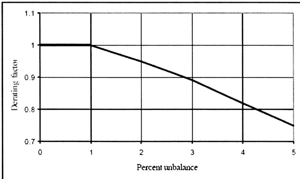
Figure 13 : Motor derating with percentage unbalance
