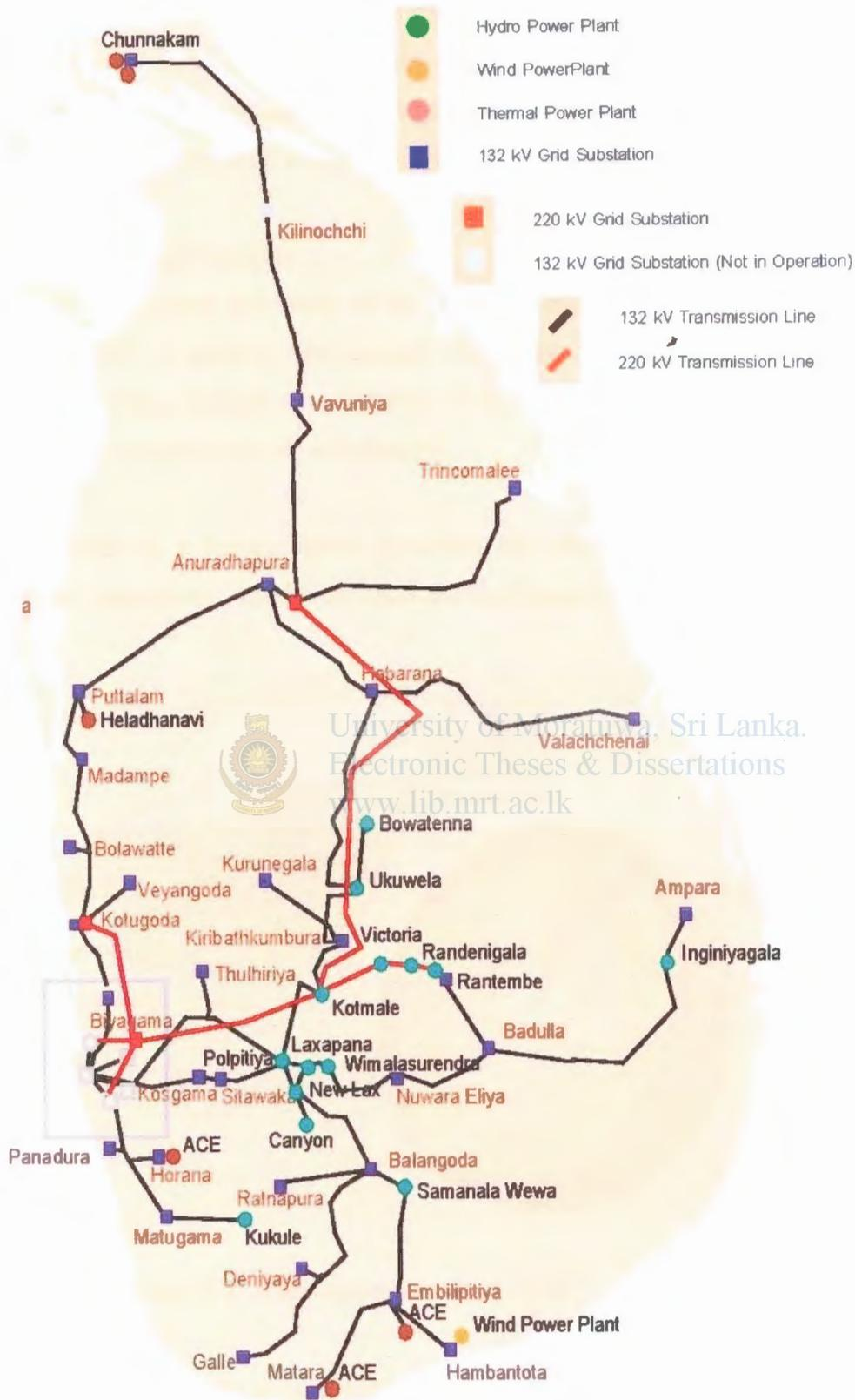
Figure 6.1 – Sri Lankan Electrical Transmission System
