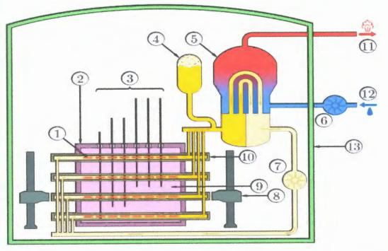
Figure 4.4 - Schematic Diagram of a CANDU reactor
