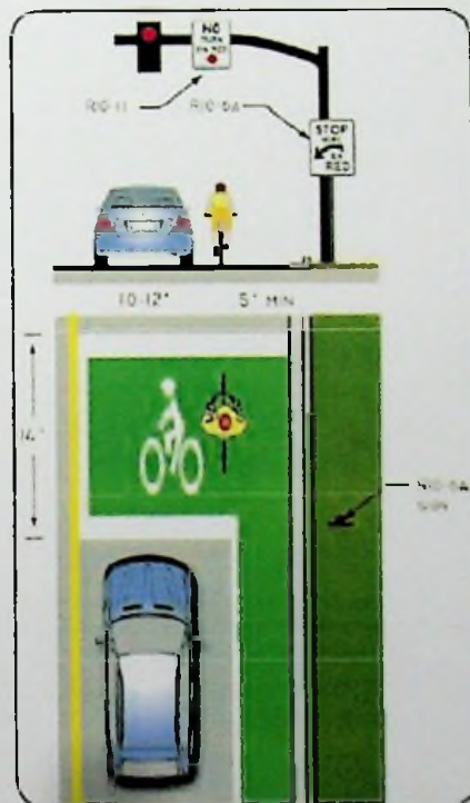
Figure.2.8 Recommended Bike Box Design
