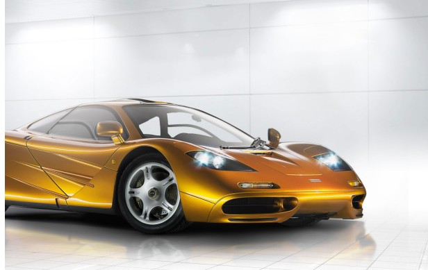
Figure 1.2: McLaren F1 - first production car with CFRP monocoque chassis (courtesy: McLaren Automotive)
