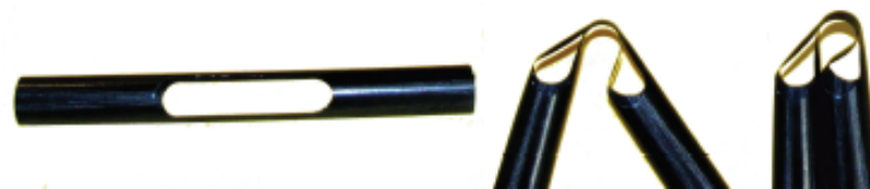
Figure 1.5: States of tape spring in self-deployment
