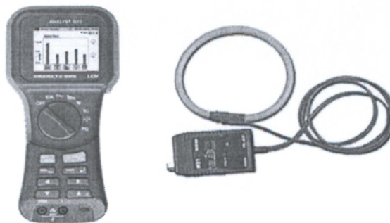
Figure 14 : Power quality analyzer with flexible current transformer
