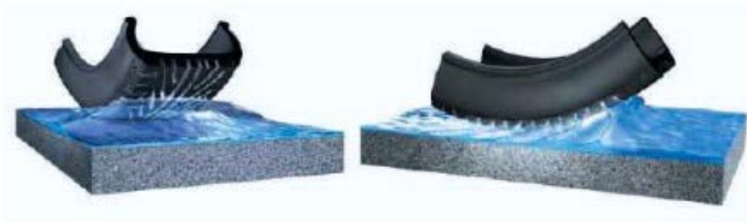
Figure 1-2 Separation between the road surface and vehicle tire (Foucard-2005)
