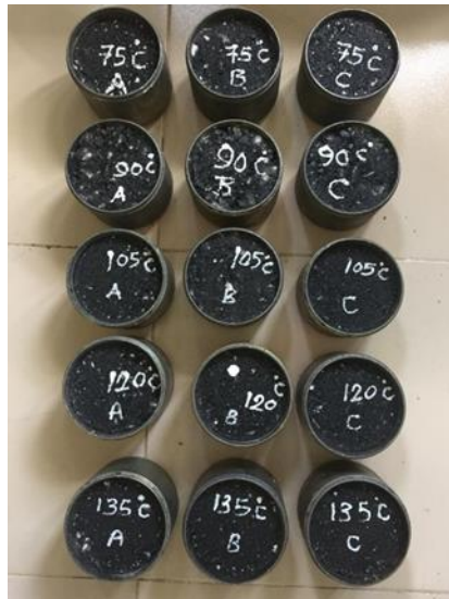
Figure 4. 1 Marshall Samples for different compaction temperature
