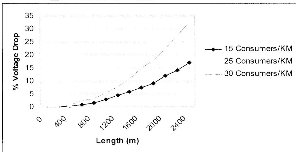
Figure 1.2.2 – Percentage Voltage Drop vs. Line Length
