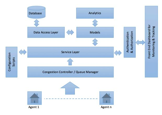
Figure 3-2 : Modular Architecture of the API
