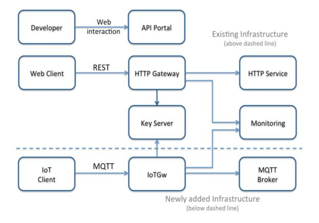
Figure 2-2 : Overall System Architecture
