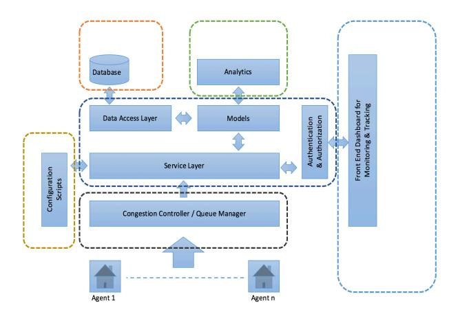
Figure 4-4 : Components level scaling architecture
