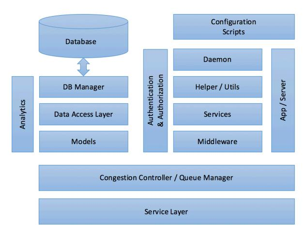
Figure 4-1 : Components diagram of API
