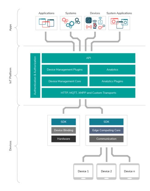
Figure 2-5 : High level System Architecture of WSO2 IoT Server
