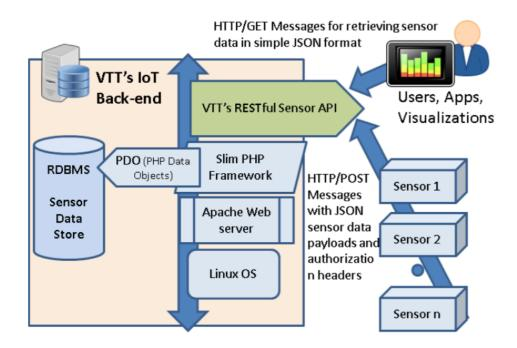
Figure 2-4 : Overview of the first PHP-based RESTful IoT Back-end prototype
