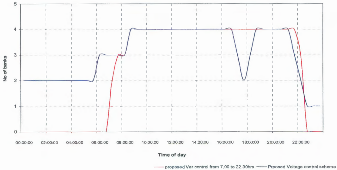
Figure: 6.7 comparison of switched banks under voltage control schemes & var control with manual off - 24 th Jan
