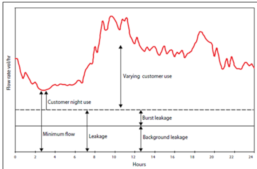
Figure 2.8 : Typical 24-hour DMA flow profile indicating MNF.
