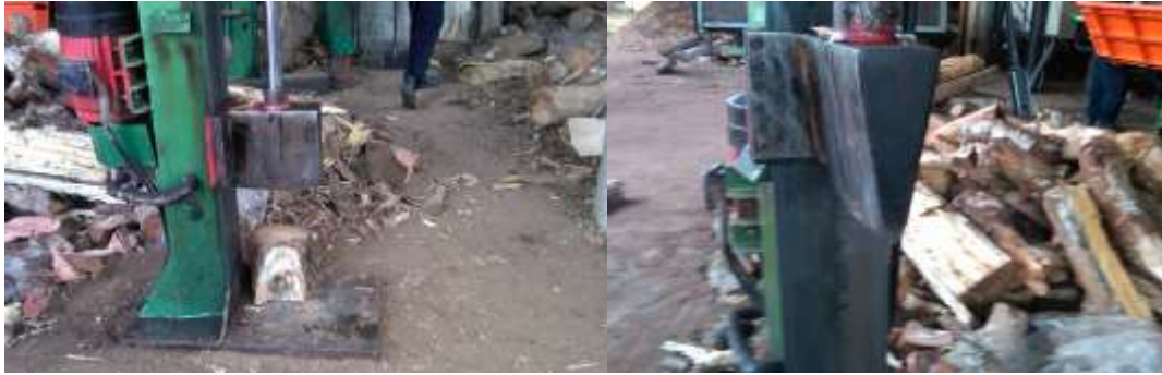
Figure 2.7: Splitter machine chopping the mixed fire wood
