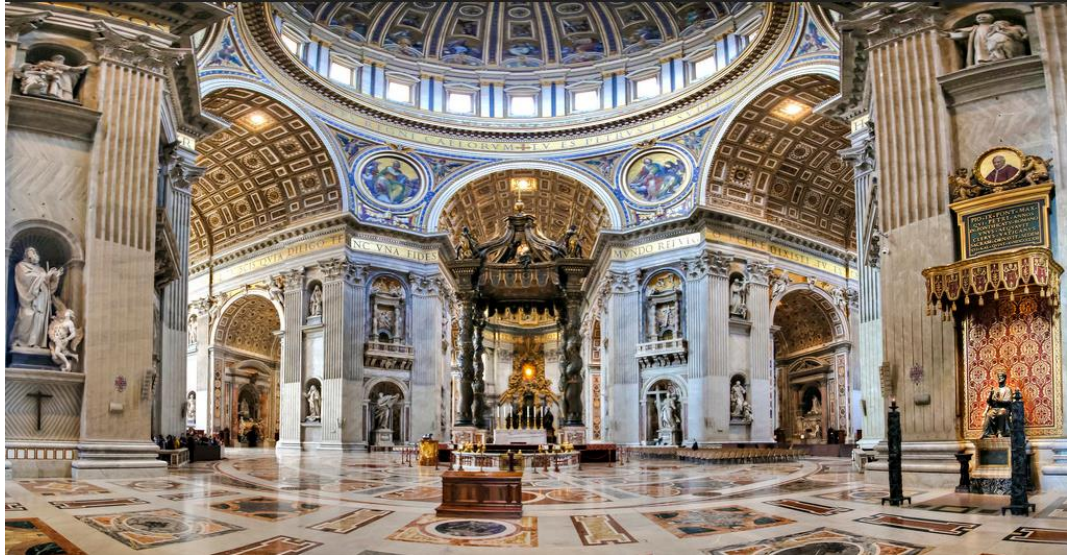
Figure 2.6: Panoramic view of St Peter's in Rome, shows barrel vaults in the transepts and the central dome. Source: Jonathan Garcla.
