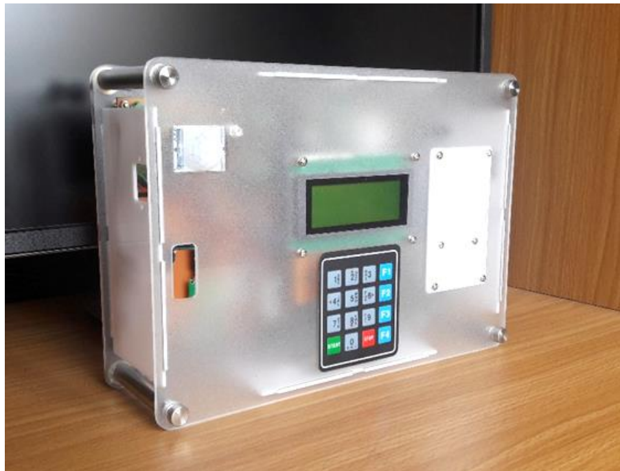
Figure 4.77: An image of the central controller
