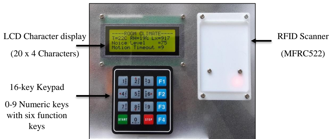
Figure 4.23: Developed inbuilt HMI on front of the IHAS central controller
