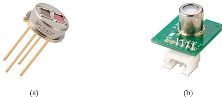
Figure 4.25: IR Thermopile sensor (a) Thermopile sensor element (b) PCB mounted thermopile sensor module
