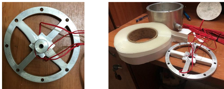
Figure 69: SB tape covered strain gauges
