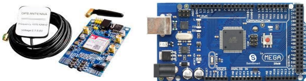
Figure 77: SIM808 GSM/GPRS/GPS module and Arduino Mega
