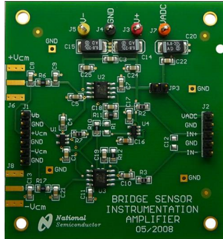
Figure 73: LMP2021MAEVAL instrumentation amplifier evaluation board
