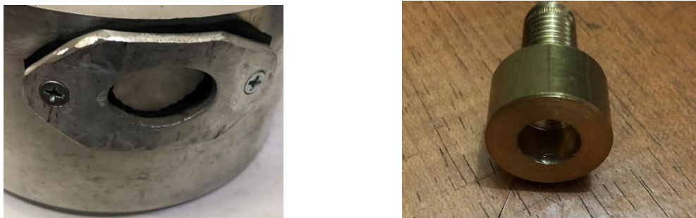
Figure 63: Water infiltration holes outer rings and cable tiding rings
