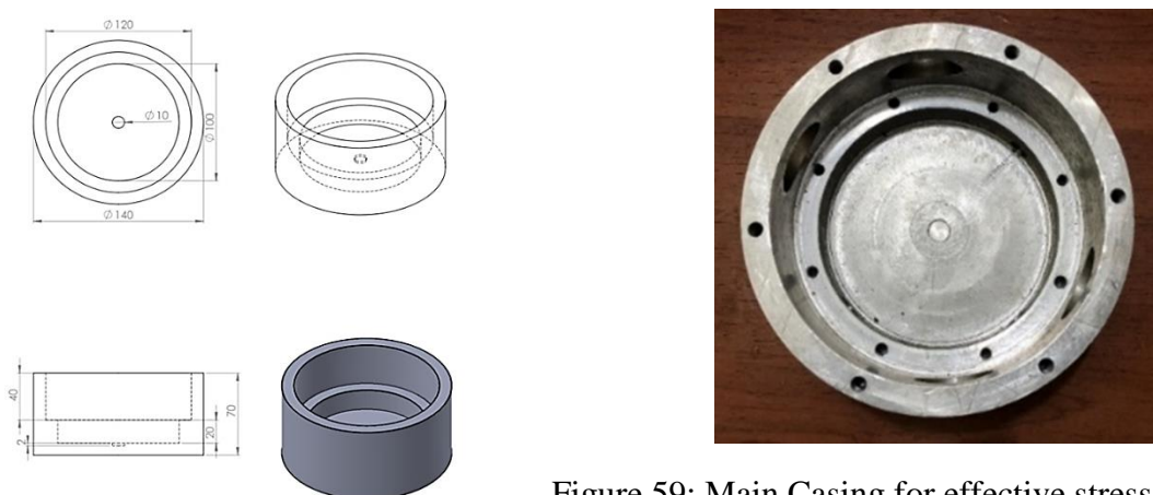
Figure 59: Main Casing for effective stress measurement
