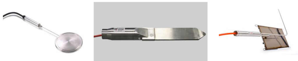
Figure 2: Earth pressure cells [6]
