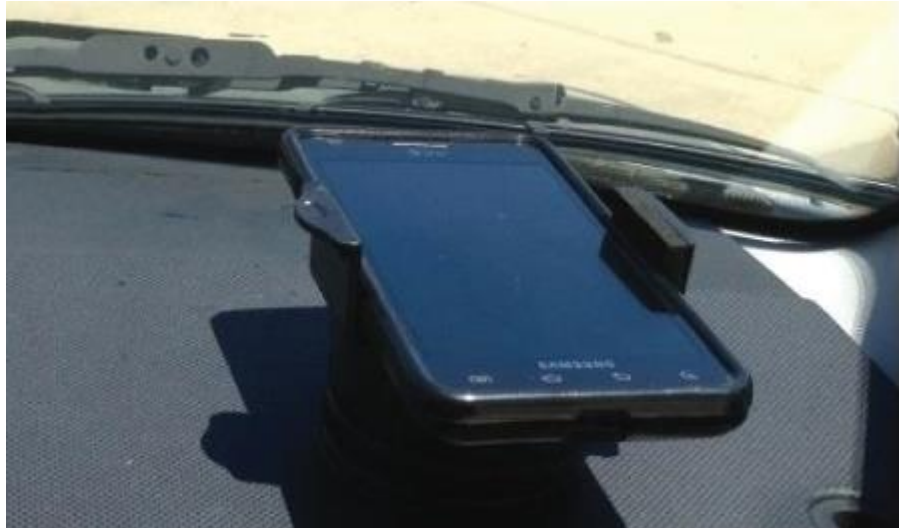
Figure 2.8: Smart phone arrangement during roughness data collection
