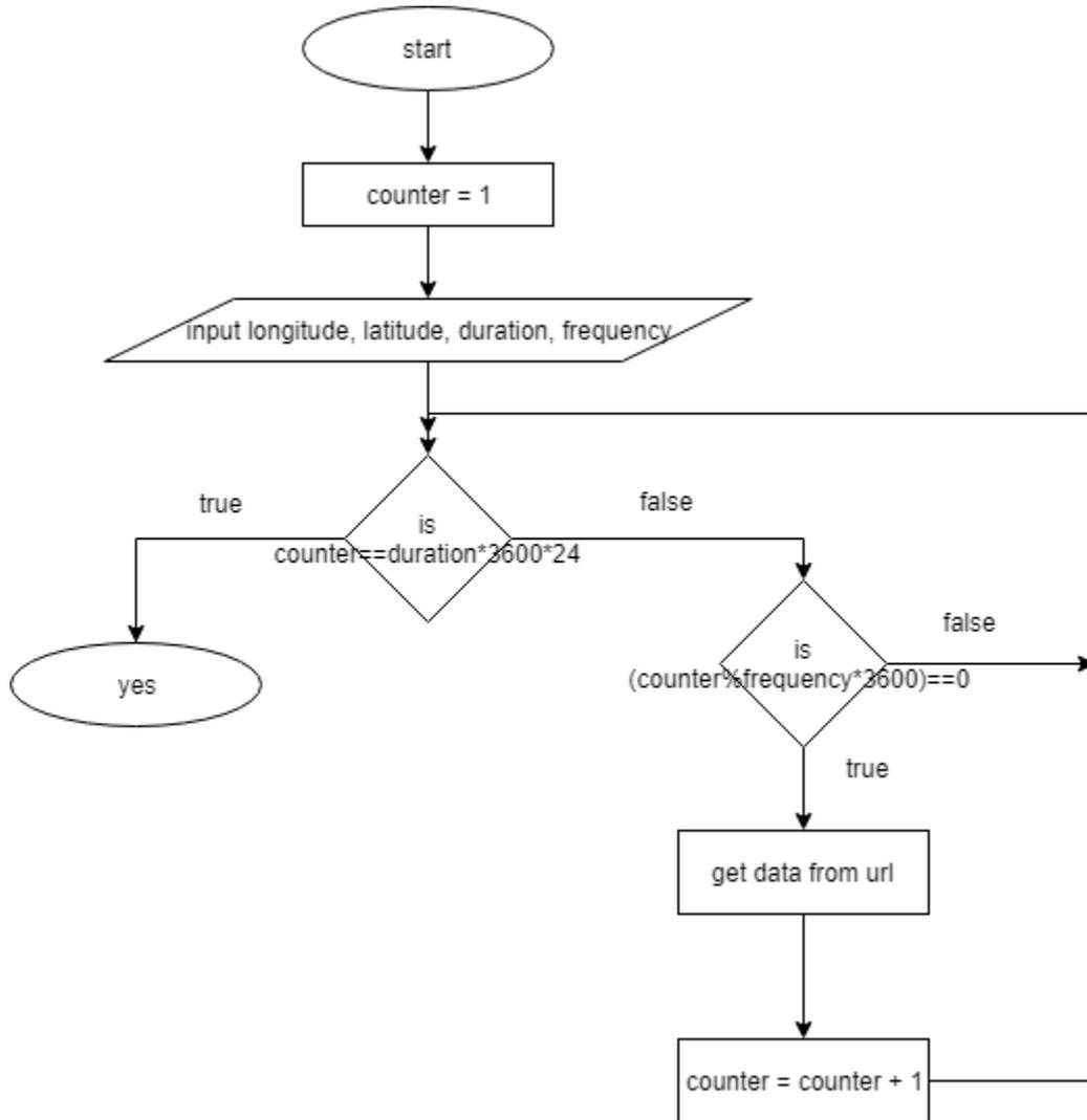
Figure 12: Flowchart of the code which are used to collect data
