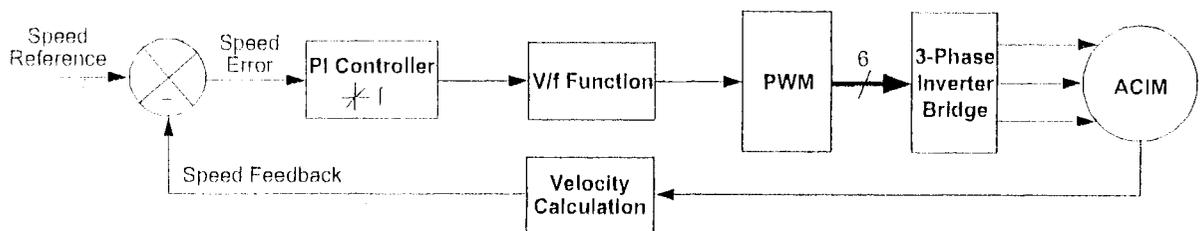
Figure 7.1 – Block diagram of VSD with feed back control
