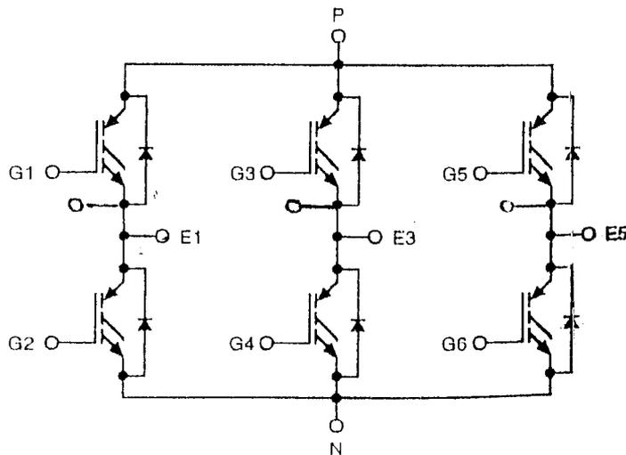
Figure 5.1 – Six-pack IGBT module with emitter Kelvins.
