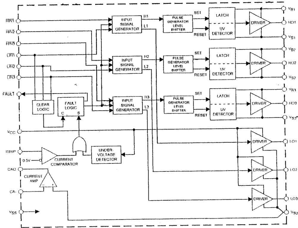
Figure 5.2 - Functional block diagram of the IR 2130
