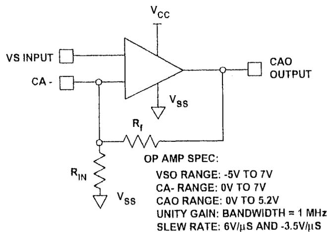
Figure 5.3 - Block diagram of the Current Sensing amplifier
